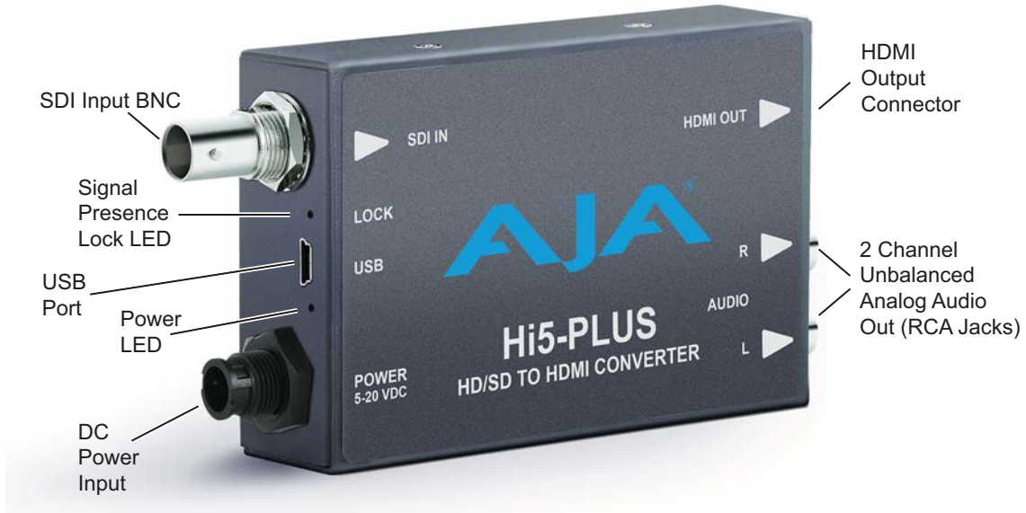
Figure 2. Hi5-Plus Converter Connections
